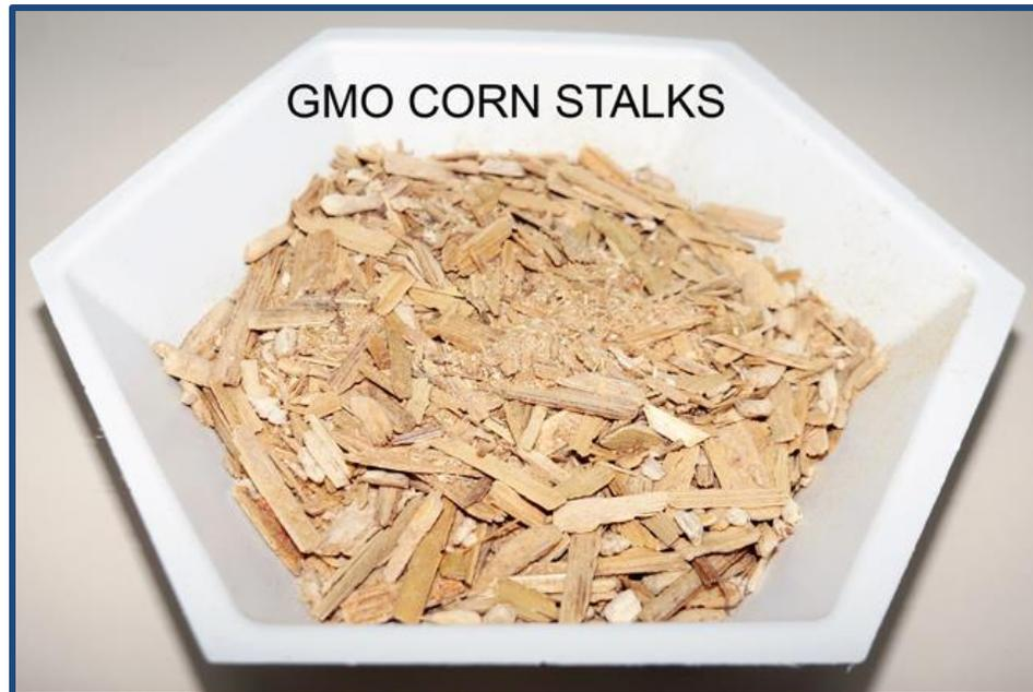
Using a precision balance, the mass of six empty, clean, and dry porcelain crucibles was determined to within 1 milligram. The mass of each was recorded and referenced as ( $M_p$ ). The crucibles were tared individually to 0 on the same balance. Approximately 1 gram (+/- 2 milligrams) of the final dried corn stalk was placed into each one. The corn stalks masses were recorded and referenced as ( $M_c$ )
